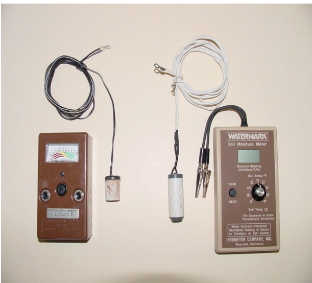
Electrical Resistance Blocks & Meters
