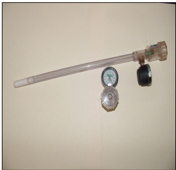
Tensiometer for Measuring Soil Water Potential
